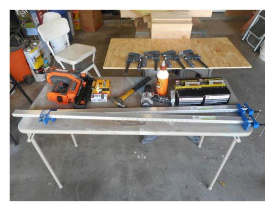
OK, first you need to start building the main frame components. You'll need 2 of these. I glue and clamp together, getting the corners square and even, then I nail.
