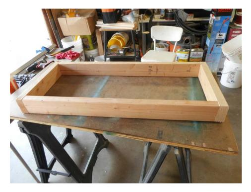
Next, you start assembling the upper and lower frames to create the main box. Look closely, you'll see where I put the glue before clamping.
