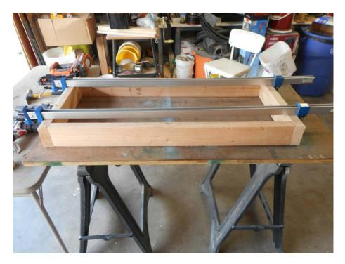
This is after the clamps are removed. It is important you notice which board is where. the short ends are on the outside!
